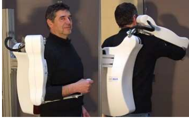
Fig. 5. ABLE 4 axis exoskeleton actuated by screw-and-cable actuators
