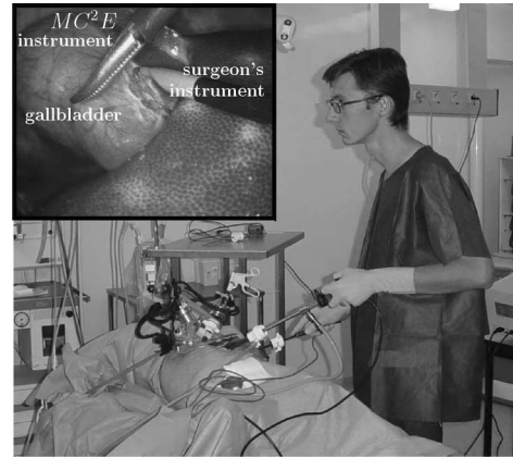
Fig. 13. MC^2E robot during an in vivo laparoscopic cholecystectomy.
