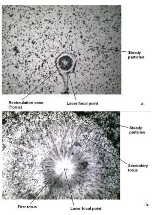
Fig. 8. Marangoni convection flows experiments, size of the image window is 1.5 x 1.1 mm². Particles are  $8-12~\mu m$  hollow glass beads. Laser: about 45 mW irradiating from below. a. 300  $\mu m$  water thickness. b. 150  $\mu m$  water thickness.
