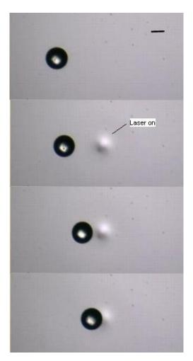
Fig. 9. Displacement of a 85  $\mu$ m glass bead in 300  $\mu$ m of water thickness using a CW IR laser, time between images 160 ms. Scale bar 50  $\mu$ m.
