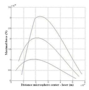
Fig. 4. Expected force profiles of three different sized particles (R=50, 100, 150  $\mu$ m). The maximum force is drawn as a function of the distance from the centre of the sphere to the laser spot.
