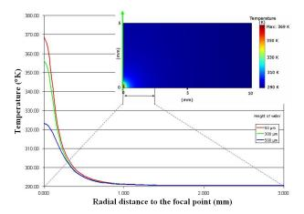
Fig. 2. a. Temperature profile resulting from a volumetric power transfer for a laser power of 66 mW at permanent state. The total Petri dish system is represented in axisymmetric geometry (green arrow is the symmetry rotation axis). Maximum temperature is on the laser spot :  $369\,^{\circ}\text{K}$  or  $96\,^{\circ}\text{C}$ . The detailed zone is marked by a double arrow. b. Detailed zone of 2 mm radius from the laser spot shows different temperature distributions along radius and height.
