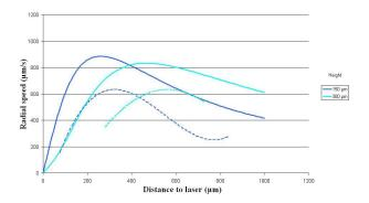
Fig. 7. Speed profiles of hollow glass microspheres (diameter 5  $\mu m)$  for different heights (150–300  $\mu m$ ). Water thickness = 1.65 mm. Solid line represent simulation results, dash lines are experimental measurements.
