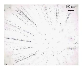
Fig. 6. Superposition of 15 images of the CMOS camera, picture shows microspheres from 2 to 20  $\mu$ m converging on the laser spot. Four example trajectories are marked by a segment. Water thickness is 1.65 mm and images have been taken in 0.6 mm height of water.
