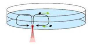
Fig. 1. Concept of micromanipulation using natural convection flows.
