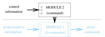
Fig. 4. During a first evolutionary stage, Module 1 is evolved. That module receives proprioceptive information through sensory cells and influence actuators through motoneurons. In a second evolutionary stage, Module 2 evolves. That module receives control information through special sensory cells called *control units* and can influence the behavior of the animat by making connections with the cells of the first module.
