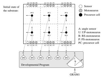
Fig. 6. Setup for the evolution of a straight locomotion controller for a sixlegged animat. The figure shows the initial positions of the sensors, motoneurons and precursor cells, as well as the structure of the developmental programs that call upon seven subprograms. JP is a call instruction that forces a cell to start reading a new subprogram. Only subprogram 6 needs to be evolved. It's organization is constrained by the GRAM1 grammar. Additional details are to be found in the text.
