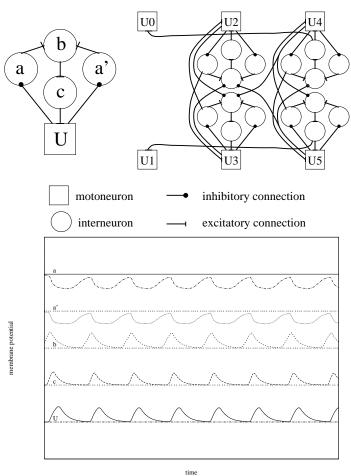
Fig. 9. Part of the circuitry that is responsible for foot-position control. A basic oscillator (Upper, Left) is copied four times within the control architecture. These oscillators are connected in such a way that the feet of adjacent legs are raised out of phase with each other (Upper, Right). When the basic oscillator is simulated in isolation, the membrane potentials of its different neurons oscillate as shown at the bottom.
