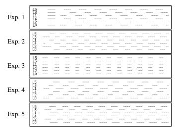
Fig. 7. Best gait in the final population for each of the five experiments. The horizontal axis represents time. A dot is plotted when the corresponding leg is raised. Legs are numbered as in Figure 6. Only the results of Experiment 2 correspond to a stable, tripod gait. All other experiments in the series led to unstable, leaping behaviors.
