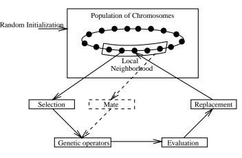
Fig. 3. The evolutionary algorithm.
