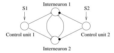
Fig. 17. A solution discovered by the evolutionary algorithm to implement a switch mechanism. Inhibitory and excitatory connections are represented as in Figure 9. In the absence of significant input, both interneurons have a low output value. Whenever S1 is presented, however, they are excited and the reciprocal excitatory connections keep their output values high. Finally, whenever S2 occurs, they are inhibited and return to their quiescent state.
