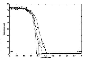
Fig. 13. The distance covered during 1000 cycles when a fixed continuous command value is applied. Each curve represents the mean distance covered in ten runs.
