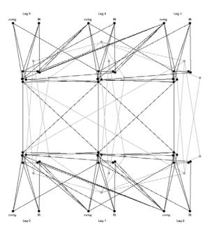
Figure 7: An example of an evolved controller. Black neurons belongs to the module controlling locomotion, gray neurons belong to the module controlling obstacle avoidance. The first controller contains 48 neurons and 82 connections; the second one contains 14 neurons and 36 connections.
