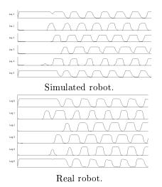
Figure 6: Comparison of leg movments in the simulated and the real robot. Both graphs show commands sent to leg swing motors. Althought the controller's outputs might have been altered by the procedure preventing over currents in the real robot, the commands actually sent to the motors, and hence the robot's overall behaviors, are qualitatively the same in simulation and in reality.
