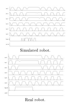
Figure 9: Leg swings in the simulated and the real robot during obstacle avoidance. When an obstacle is detected at the right (Right IR) of the robot, the three legs on its left (Leg0, Leg1, Leg2) are temporarily blocked.
