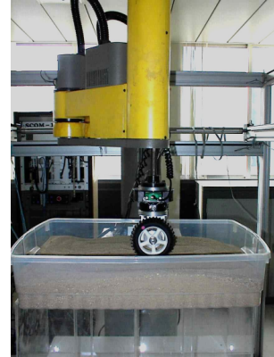
Figure 3: Testbed of wheel-sand interaction with a Scara manipulator.
