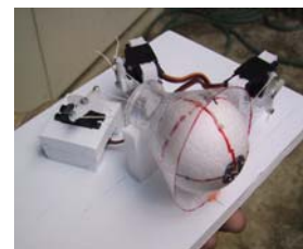
Figure 16. An eye equipped with a camera and a log-polar sensor, which is actuated by three motors. The whole device obeys the Listing's law (von Helmholtz, 1955).
