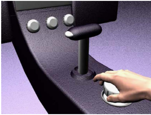
Fig. 1 Artist's view of a multi-function haptic knob for vehicular instrument control
