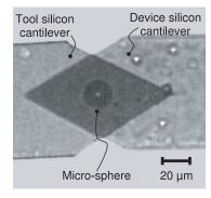
Fig. 5. Cantilever/sphere/cantilever contact.
