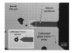
Fig. 4. Cantilever length and width measurements,  $L=450\mu m$  and  $l=90\mu m$ .
