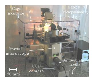
Fig. 1. The FBM experimental setup overview.
