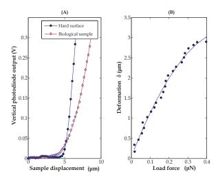
Fig. 7. (A) Experimental data of the photodiode output as function of the sample displacement performed on both single EpH cell and hard surface. (B) Experimental curve of the sample deformation  $\delta$  as function of the applied load by the cantilever.
