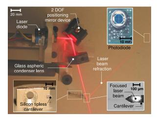
Fig. 2. The mechanical sensing unit.
