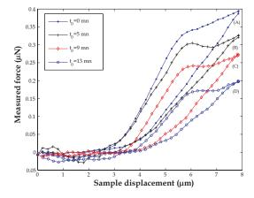
Fig. 8. Evolution of the measured force as a function of the sample displacement for different elapsed times  $t_0=0,5,9$  and  $13\ mn$ .
