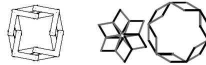
Fig. 4. Expanding "4-gon" and "6-gon" based on Hoberman design
