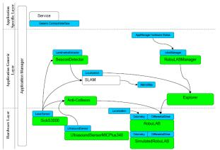
Fig 4: RobuBOX services architecture example for an explorer robot creating a metric map of its environment
