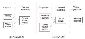
Fig. 8. The autonomous navigation process.
