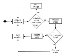
Fig. 1. Overall process diagram (see text for details).
