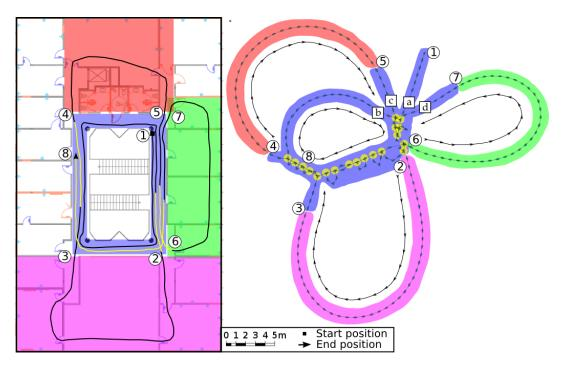
Fig. 5. Floor plan of the travelled environment superimposed with the trajectory of the camera (left part of the figure) and corresponding topological map (right part of the figure). The graph layout is performed using a simple "spring-mass" model [19]. See text for details.
