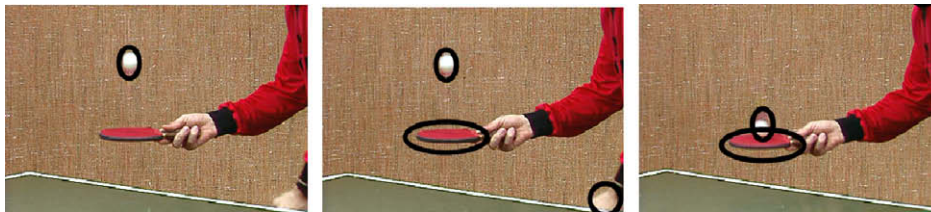
Fig. 8. Results on the “Tennis” sequence: from left to right: 1. detection of the ball with a quasi null motion (top of the parabola of the trajectory); 2. the ball is accelerating: the racket, the ball and the hand are well detected; and 3. contact between the ball and the racket, two classes are still detected.
