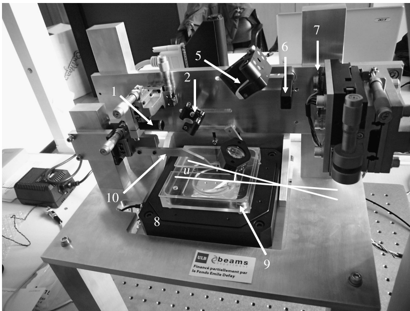
Figure 6. In addition to Fig. 5, we can see in this figure the nano-positioning stage (8), the environmental box (9) and the part on which the cantilever is glued (10). The angle \mu is the angle between the substrate to be placed on the bottom of the environmental box and the cantilever (4, not shown here).
