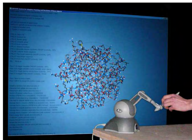
Fig. 6. The HIV molecule and its inhibitors, 848 degrees of freedom. A haptic device is used to control the inhibitors and to feel the interactions with the HIV molecule.
