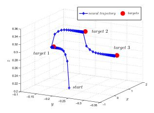
Fig. 7. "Neural" trajectory (blue) of the end-effector, reaching a target (red) which changes unpredictably. The shape of each trajectory is determined by the cost function  $\mathcal{J}$  and its parameters.
