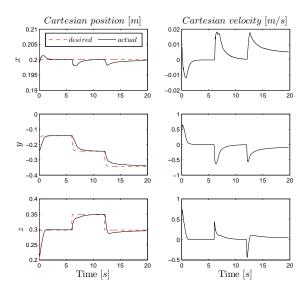
Fig. 8. Cartesian positions and velocities of the end-effector during the movements in Fig. 7. It is worth noting the different velocity profiles (e.g.  $\dot{y}, \dot{z}$ ) due to the different parameters of the cost function.
