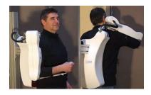
Fig. 5. ABLE 4 axis exoskeleton actuated by screw-and-cable actuators a shoulder spherical arrangement made with 3 coincident axes and a 1 DoF pivot elbow. The forearm, terminated by a handle, is not actuated. Its kinematics is sketched in Figure 6. Most of the technological originality of ABLE comes from
