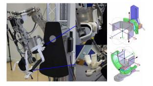
Fig. 11. The two fixations on the exoskeleton
