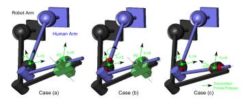
Fig. 8. Schematic of possibilities for coupling ABLE to an human arm. Case (a): ball joint alone at  $P_1$  and ball joint on 2 slides at  $P_2$ ; case (b): Universal joint + 1slide (in red) at  $P_1$  and ball joint on 2 slides at  $P_2$ ; case (c) Ball joints with slides (in red) at both  $P_1$  and  $P_2$ .
