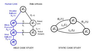
Fig. 7. Schematic of the ABLE and human arm coupling
