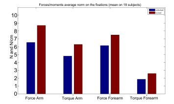
Fig. 13. Forces/torques average norm on the fixations (mean on 18 subjects) Blue unlocked and red locked
