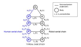
Fig. 1. Schematic of two serial chains parallel coupling
