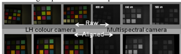
Fig. 2 Sample images acquired by the left stereo camera and multispectral camera showing the colour chart in different positions at 500, 640 and 680 nm before (raw) and after alignment.
