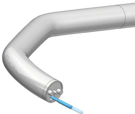
Fig. 1 Schematic illustrating an articulating endoscope (grey) and a typical confocal laser endomicroscopy imaging probe (blue). Maintaining a constant tissue contact force with such probes manually is challenging during endoscopic optical biopsy
