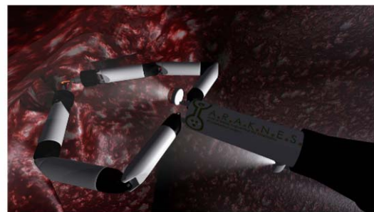
Fig. 1 3D concept of the bimanual robot for Single Port Laparoscopy.
