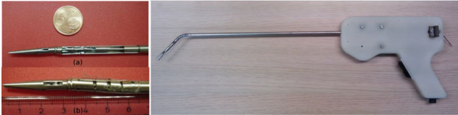
Fig. 6. (a) The two developed end-effectors, (b) Photograph of one of the developed prototypes
