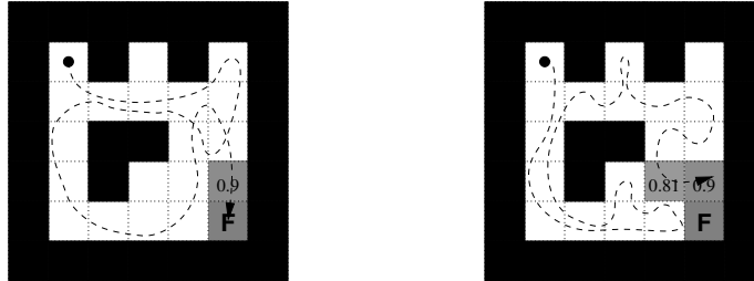
Figure 2.1. Q-learning: first and second trial. One can see that, all values being initially null, the propagation of non-null values does not start until the agent finds the reward source for the first time, and only progresses once per trial.
