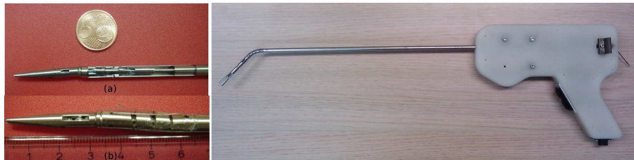
Fig. 6. (a) The two developed end-effectors, (b) Photograph of one of the developed prototypes
