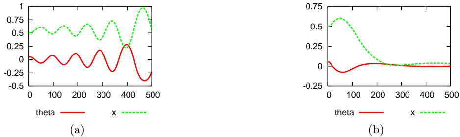
Fig. 11 Typical behaviors of the position x of the cart and of the value of \vartheta for a 100.858 fitness (a) and a 100.965 fitness (b). At t = 0 , the poles starts from \vartheta = 0.01 rad and x = 0.5 m. The controller has to drive the pole to \vartheta = 0 rad and x = 0 m. Controller (a) avoids the pole from falling during this evaluation, but the increasing amplitude suggests an imminent fall.
