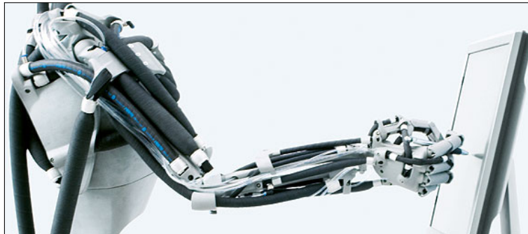
Figure 7.4: Festo arm with pneumatic actuation.
