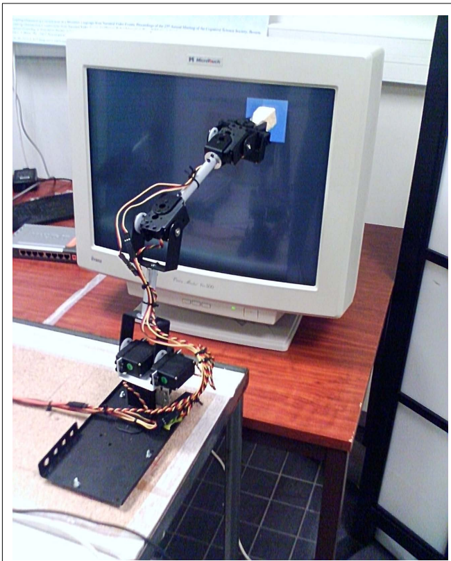
FIGURE 1 | Lynxmotion SES robotic arm in front of a touch screen used for Experiment 1. The screen is perceived by a webcam. The arm has a gripper with a sponge surrounded by aluminum connected to the ground. This produces a static current when contacting the screen and enables the screen to detect when and where the robot touches it. This setup allows us to test the robot in the same experimental conditions as the non-human primate subjects in our previous studies (Amiez et al., 2006; Quilodran et al., 2008).
