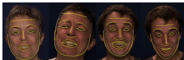
Fig. 4. AAM results on test images highlighting accurate localizations on mouth or chin and localization problems on eyebrows
