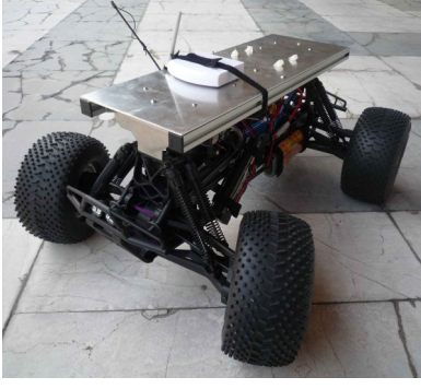
Fig. 2. Mobile robot “fastBot 2”, for which the controller is designed.
