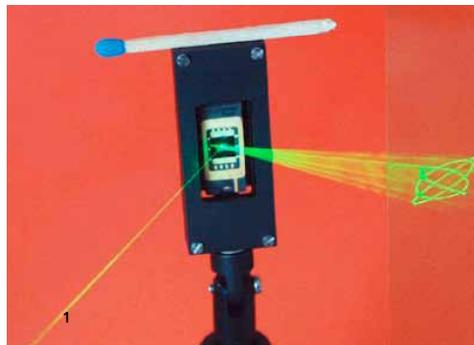
FIGURE 2.11 – Micro miroir scanner chez IPMS Fraunhofer
