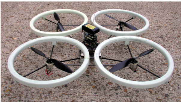
Fig. 2. X4-flyer: quadrotor developed by CEA-List.
