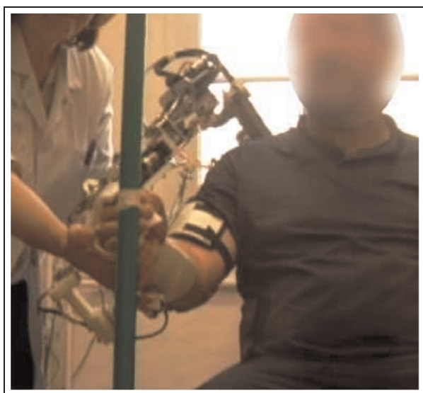
Figure 4. Arm manipulation of an hemiplegic patient by a physical therapist and an upper-limb robotic exoskeleton, performed at the Raymon Poincaré Hospital, Garches, France. Such tasks require a complex sensorimotor coordination strategy between the physiotherapist and the training patient. Reproduced with kind permission from the IEEE (Crocher, Sahbani, Robertson, Roby-Brami, and Morel, 2012).
