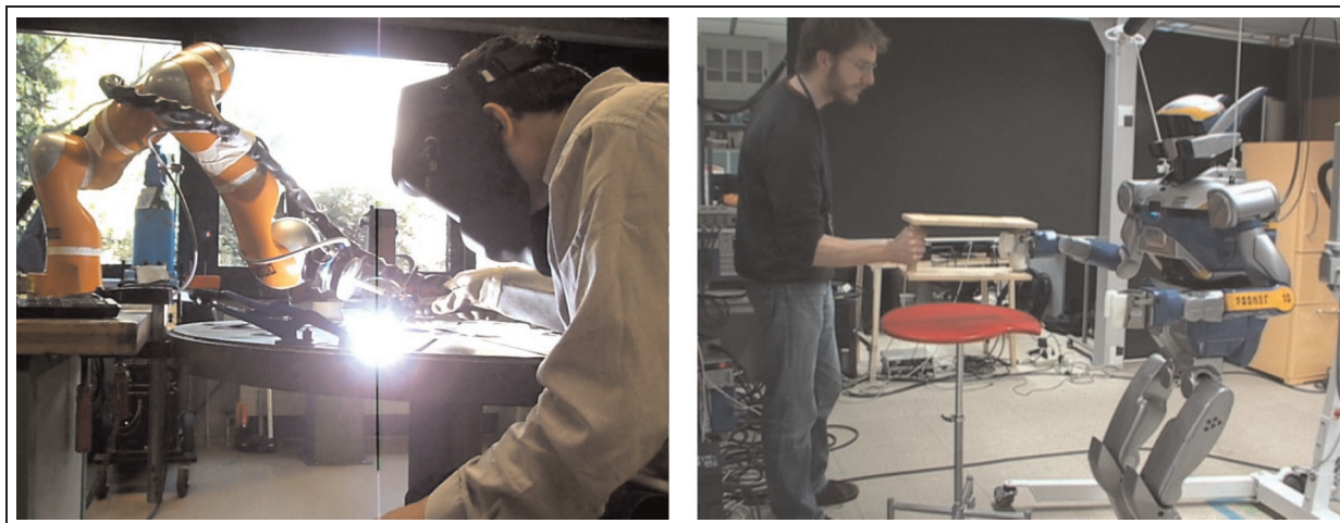
Figure 2. Human–robot joint motor action. Left: KUKA(r) LWR robot used for arc welding (with permission from Mustafa Suphi Erden conducting research at LASA, EPFL). Right: HRP2 robot used by Evrard & Kheddar (2009b). Reproduced with kind permission from the IEEE (Evrard & Kheddar, 2009b)
