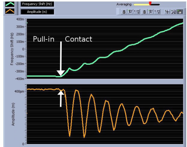
Fig. 10. Shape of the frequency shift (upper curve) and amplitude (lower curve), spanning 1 second, upon entering into contact with a surface (Nanonis software). Frequency shifts data starts increasing towards its value measured by the pre-amplifier. Amplitude oscillates from a second order response as it is regulated by the PLL and AGC.
