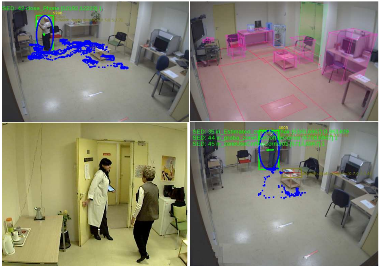
Figure 6.17: Activity detection evaluated on Health care videos. The top left image illustrates the recognition of the primitive state ‘close-Phone’, the right bottom image illustrates the recognition of the primitive state ‘inside-zone-coffeeCorner’ and the primitive event ‘change-zone-reading-to-coffeeCorner’.
