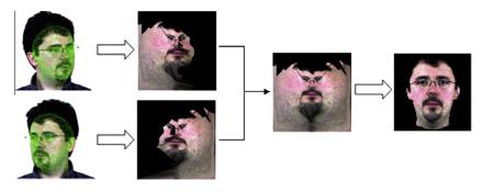
Fig. 6. Pose and shape estimation, texture map extraction, fusion and frontal view generation.
