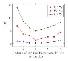
**Fig. 23.** FRR performances when integrating information over time, for three values of FAR. The value on the *x*-axis corresponds to the number of frames used for the estimation: the first value is the result using only the first frame, the following are the outputs using the video from time 1 to *i*, with our particle filter based method.
