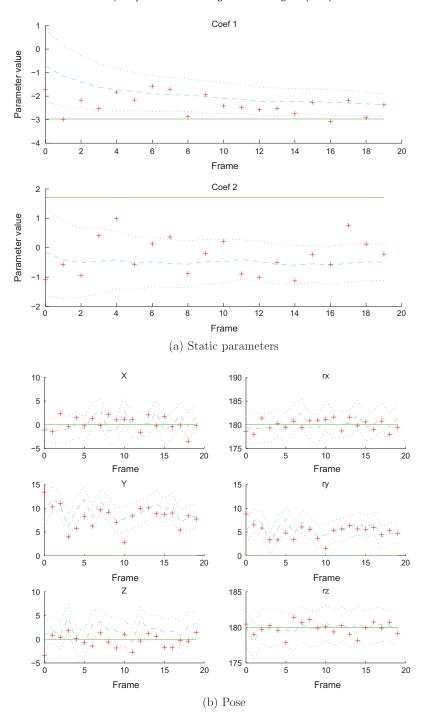
Fig. 11. Example of non-convergence of the filter towards the ground truth values with unknown pose and noisy observations. N = 2500 particles are used, and artificial moves are Gaussian noise with adaptive covariance.
