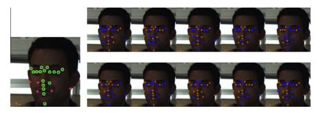
**Fig. 5.** Left image: initial detections. The red crosses (resp. the green circles) are detections with a confidence below 0.5 (resp. above 0.5). Right images: point sampling for ten particles. The orange crosses (resp. blue circles) are points which are rejected (resp. kept) for the current particle. (For interpretation of the references to color in this figure legend, the reader is referred to the web version of this article.)
