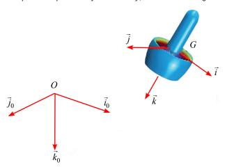
Figure 1- Attitude represents the orientation of body frame  $\mathcal{B} = \left\{O; \vec{i}, \vec{j}, \vec{k}\right\}$  w.r.t. inertial frame  $\mathcal{I} = \left\{O; \vec{i}_o, \vec{j}_o, \vec{k}_o\right\}$
