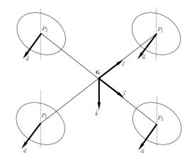
Fig. 2. Sketch representation of a quadrotor with thrust tilting capability.
