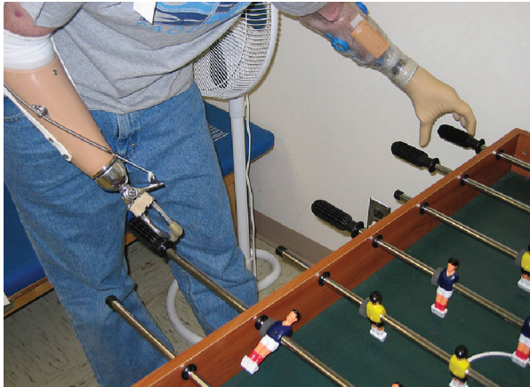
FIGURE 2. A soldier in the U.S. Army plays foosball with two prosthetic limbs: one mechanical (right arm) and one myoelectric (left arm). Courtesy of the U.S. Army, by Walter Reed photographers.
