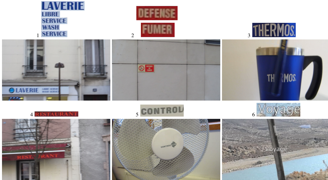
Figure 4: Our challenging video sequences. 1-2: motion blur, 3-4: partial occlusion, 5: rotation, 6: cluttered background. Zoom on text models to track (extracting from the first frame) are given above each frame.
