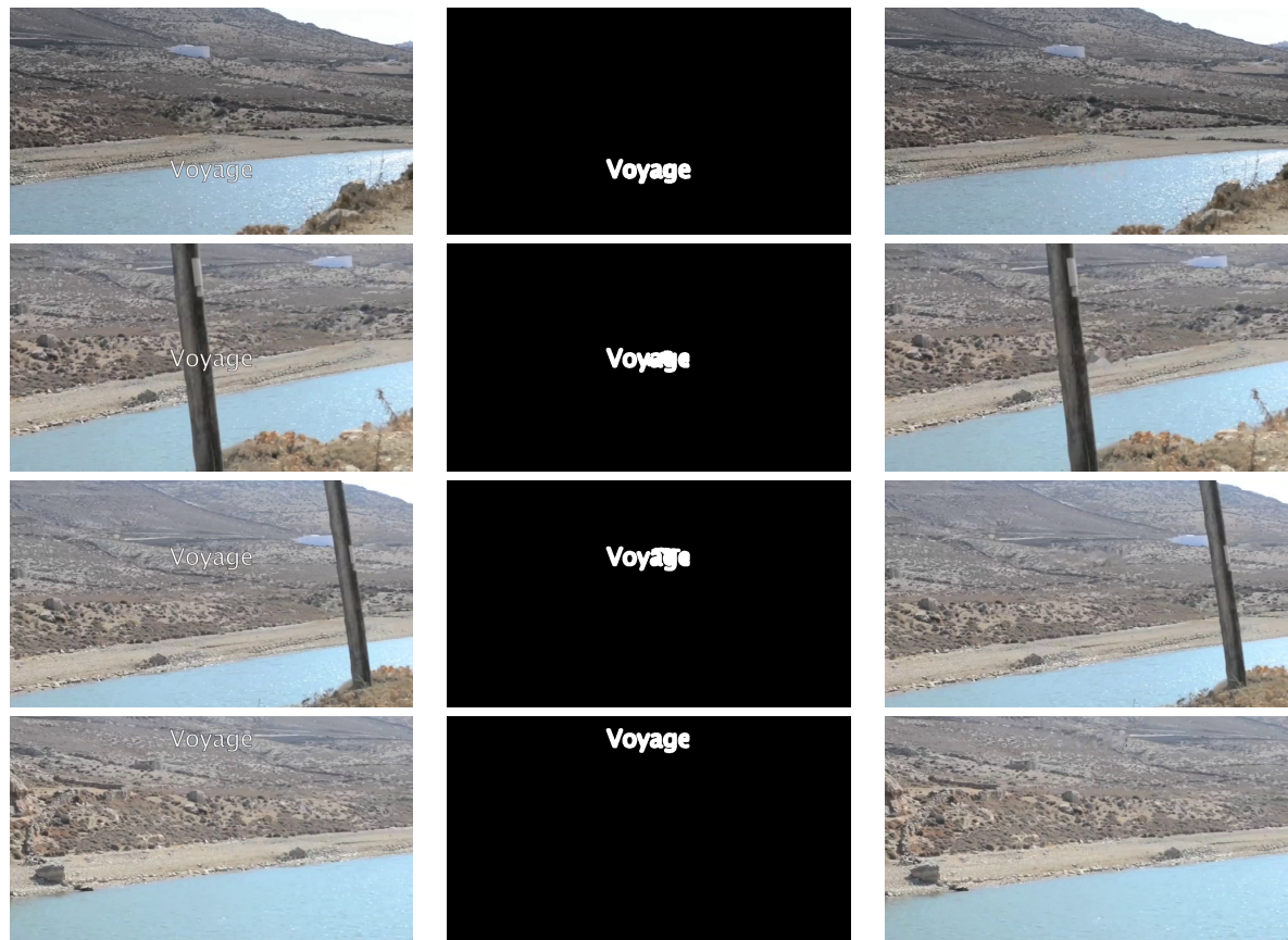
Figure 5: Example of application of our text tracker. First column presents a series of frames (33, 68, 96, 136) with embedded text. Second column gives binarized text area provided by a tracking and binarization process. Third column shows results of “inpainted” frames.
