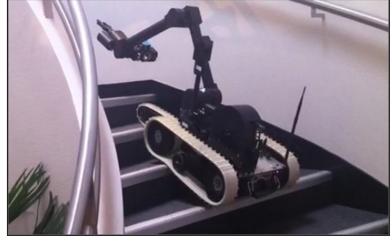
Fig. 1. A Cameleon EOD , a tracked mobile robot from Eca Robotics [13]
