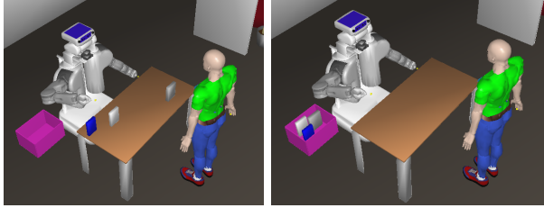
Fig. 2. The Robot and the human partner are facing the table. One tape is on human side, two tapes and the trashbin are on robot side. At left, the initial state. At right, the final state.
