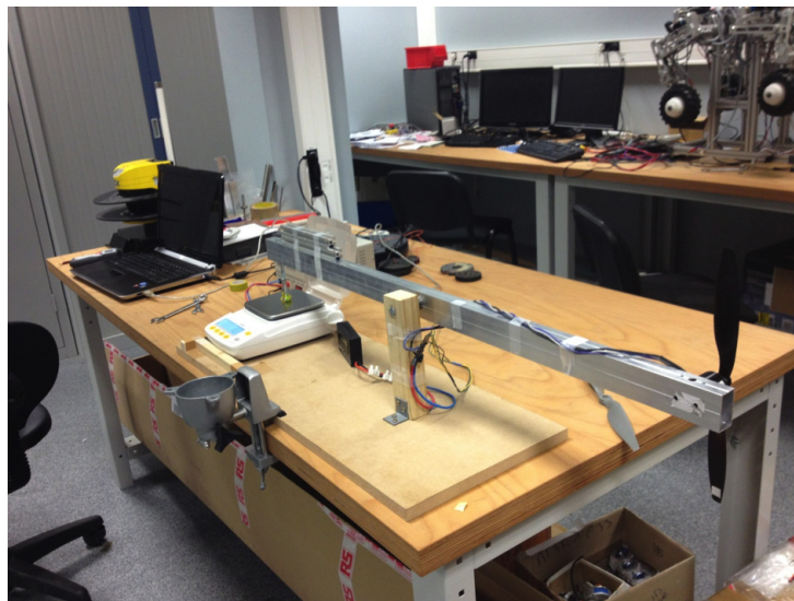
Figure B.3: Experimental setup of our static test bench for torque measurement
