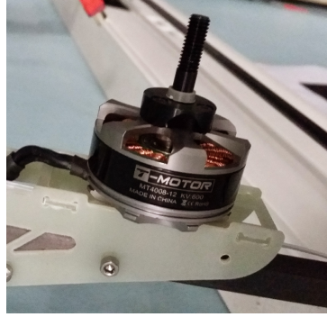
Figure 4.5: Motor mounting on the UAV frame
