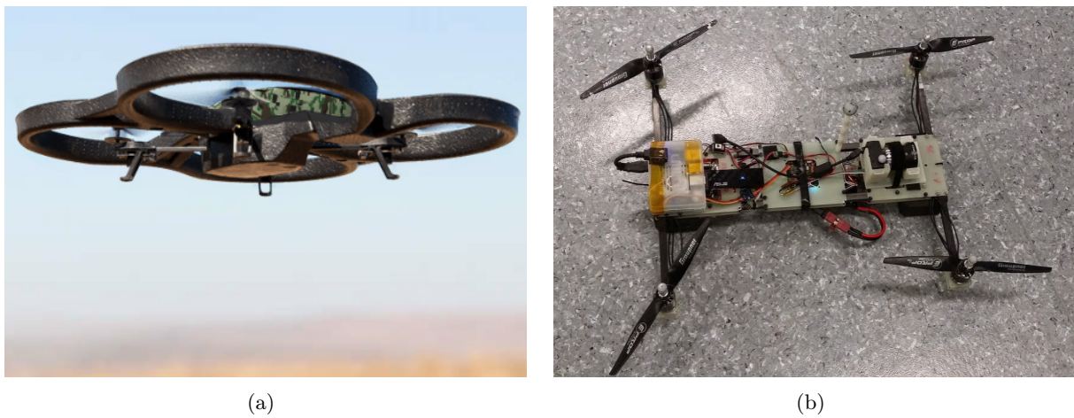
Figure 1.11: Some examples of mini quadrotors: (a) Parrot AR.Drone 2.0 ( parrot.com ) and (b) Our ISIR Prototype
