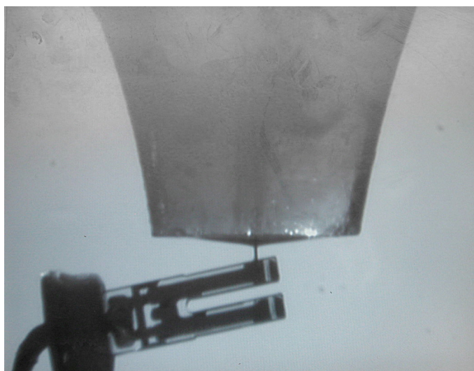
Figure 2.5 - Direct etching of a tip on a tuning fork.
