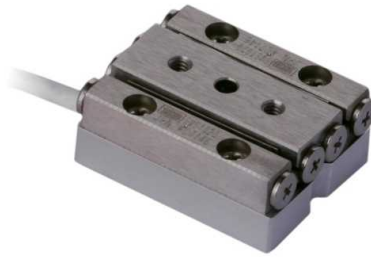
Figure 4.1 - Stick-slip piezoelectric actuator component (SLC1720) of the Smaract manipulation system, dimensions 22 \times 17 \times 8.5 mm.
