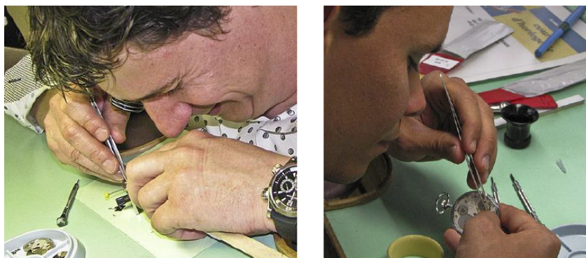
Figure 4.9: The second typical gesture to use tweezers in watchmaking process.
