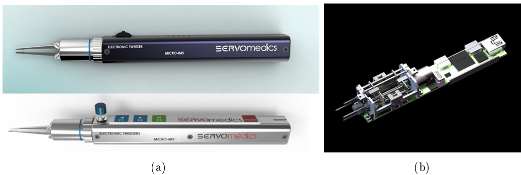
Figure 4.2: Servomedics electronic tweezers [SERVOMEDICS 2015]: (a) The blue model (shown above) is a high precision tweezers for laboratory applications; the white model (shown below) is dedicated to surgery. (b) Anatomy of a future tweezers concept: it incorporates 5 servomotors with magnetic encoders, a 32 bits microprocessor and communication network.
