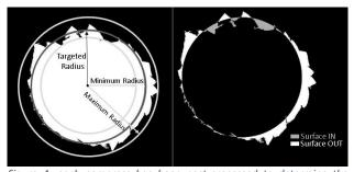
Figure 4: each compress has been post-processed to determine the minimum and maximum radius and the interior and exterior surfaces
