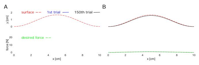
Fig. 3. Simulation of haptic exploration of a surface of unknown shape and mechanical properties along x-axis with the controller of [14] (A) and with the new controller (B). The top panels show the robot's trajectory and the bottom panels the contact force. The new controller avoids large interaction force and enables to regulate the force, while identifying the interaction surface geometry.
