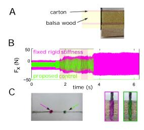
Fig. 7. Drilling heterogeneous material. A: Section of the block. B: Comparison of vibrations level in the horizontal plane transmitted to the robot structure (read on the force sensor) when using a driller speed generating "resonance", without (red) and with (green) stiffness adaptation. C: Adapting impedance reduced the hole carried out by the drill.
