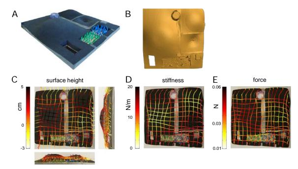
Fig. 8. Haptic exploration of a surface with unknown geometry and mechanics. From left to right: A: Photo of the test surface that was used for the pilot experiment. B: 3D scan of the test surface. C: Volume identified by the robot while scanning the surface along the line superimposed on top and two lateral views. D: End point stiffness during exploration. E: Nearly constant interaction force of about 0.05N maintained on the surface.
