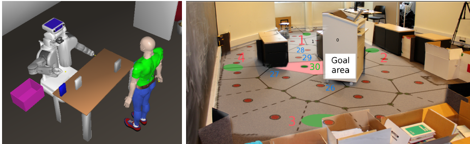
Fig. 3. (Left) Human-Robot Interaction task tested in [60]: the human and the robot collaborate to put all boxes in a trashbin. (Right) Navigation task autonomously mapped and discretized by the robot during exploration [60, 50]. The red area indicates the goal location whereas the green areas indicate starting locations of the robot. Red numbers are starting location indexes; blue numbers are some states where some changes in the configuration of the environment can occur. Adapted from [60].
