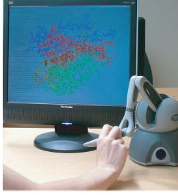
Fig. 1. Manipulation of a tetraethylammonium (TEA) around a potassium channel (KcsA), 1428 degrees of freedom.
