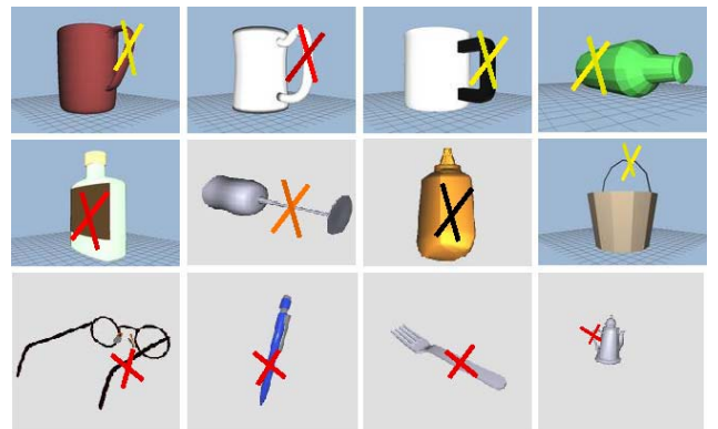
Fig. 8. Some real objects on which the algorithm was tested, the grasping component is marked with a cross
